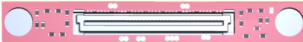
Bottom View with B2B connector (J1)
