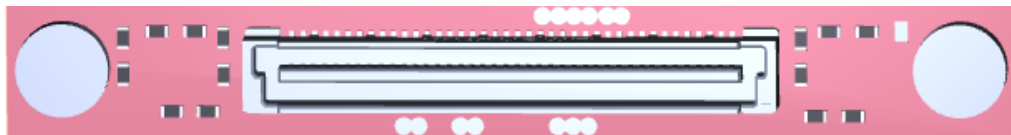
Bottom View with B2B connector (J2)
